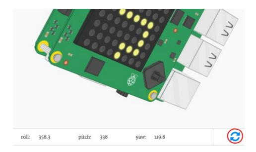
Press the reset button to put the Sense HAT back to the starting position when you've finished testing.
