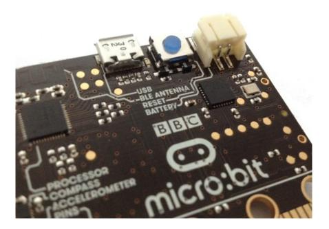
You should now see your image on the micro:bit. If you prefer, you can remove the USB cable from your micro:bit, and attach the battery. The program will be saved on the micro:bit.
